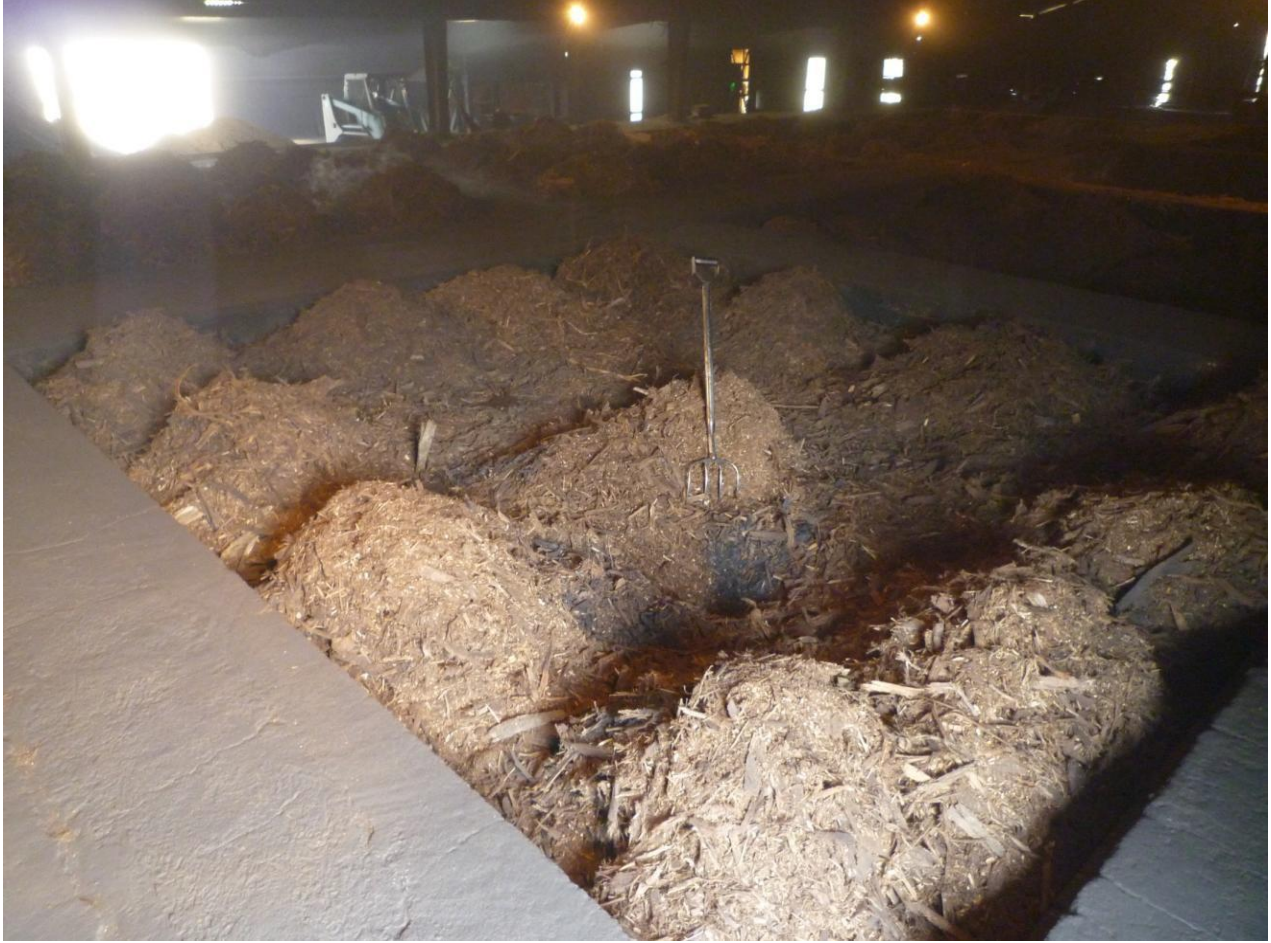
Figure 1. Dry distillation of bark from broadleaf trees in a flat kiln. New barks (brown) are placed above the previously carbonized barks (black); smoke is absorbed by the smoke flue at the bottom.
