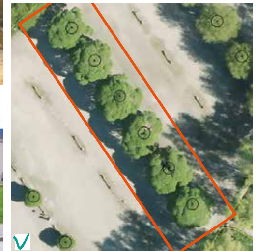
The fence is placed beyond the trees' drip line. No materials may be stored inside the fence. No traffic or machinery may move inside the fence.
