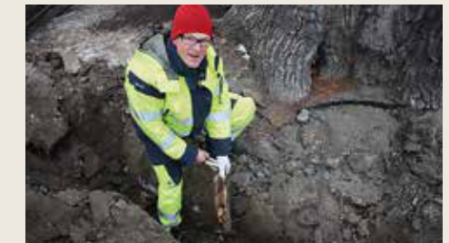
Sample excavation of oak on Fiskartorpsvägen - rotting and dead coarse roots were discovered at 60-70 cm depth.
