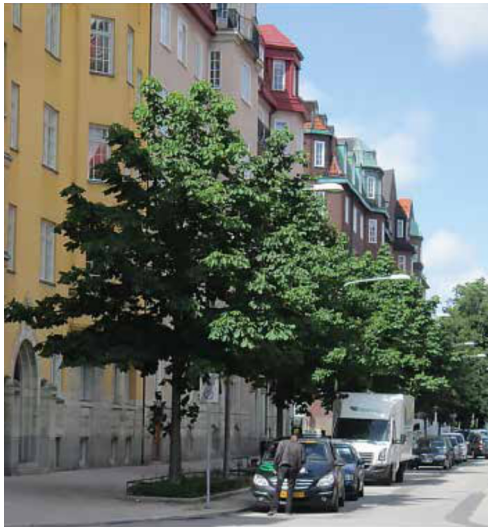
Newly planted trees with structural soil after about eight growing seasons – Erik Dahlbergsallén.
